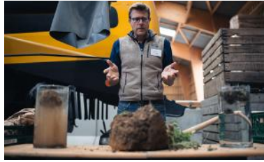
Operating a Slake Test to compare the structure between two types of soil. The regenerative agriculture sample on the right shows better soil structure and is less prone to erosion.
