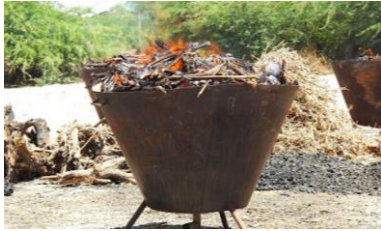
The 'Kon-Tiki Kiln' converts invasive wood into biochar
